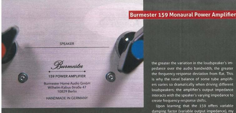
the amplifier's output impedance to the loudspeaker's load impedance. Technically, the speaker cable's resistance should be added to the equation. But ignoring the speaker cable's resistance for now, if we have a power amplifier with an output impedance of 0.1 ohms driving a loudspeaker with a nominal impedance of 8 ohms, the damping factor is 80 (8 divided by 0.1).
