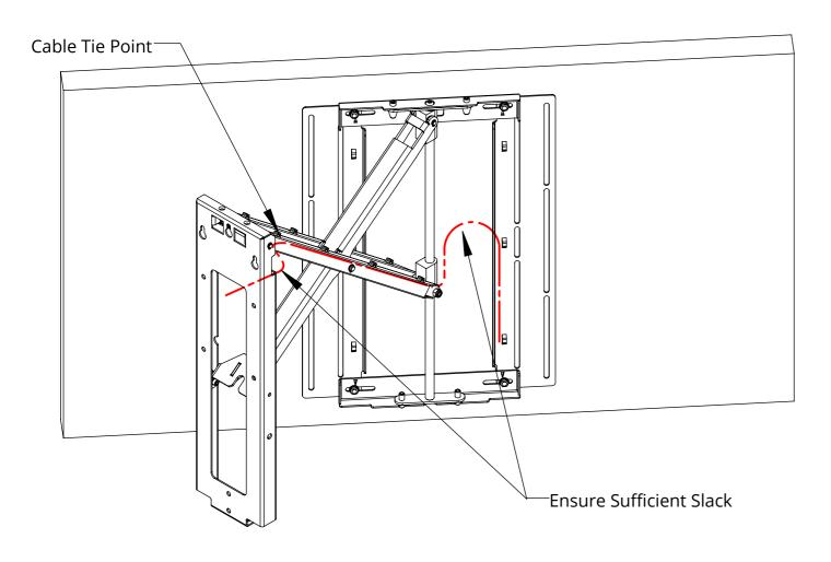
Wall sockets should be ideally placed as shown outside of the bracket footprint to maximise space for cable routing
