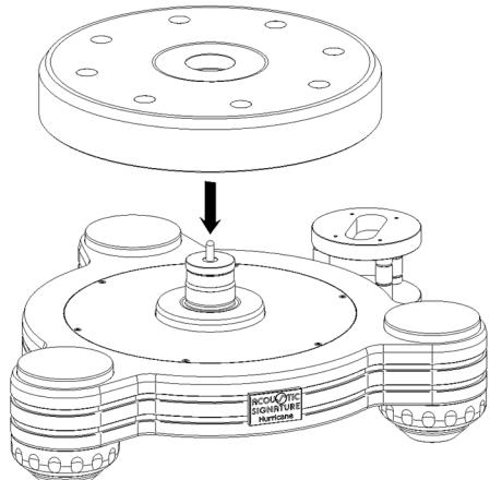
Place the platter carefully on top of the subplatter as shown in the picture above. Make sure that both cones are free of any dirt. This may affect the precise run of your turntable.
