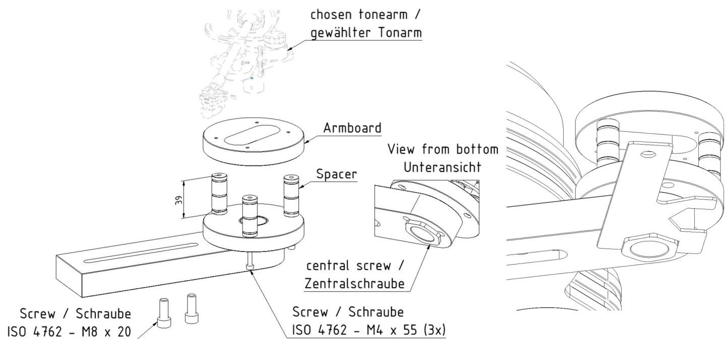
Use the delivered special wrench to handle the central screw.
