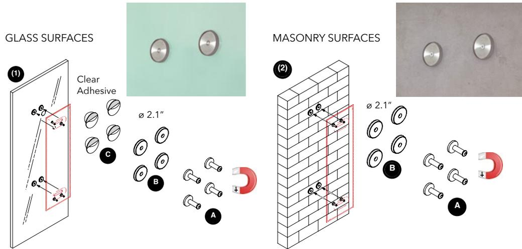
\* For ultimate bond allow 24 hours for adhesive tape to cure before attaching panels to glass mounted plates.
