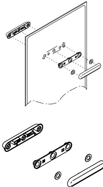
Set of connection brackets and front caps to be used when mounting MITESCO panels. Complete kit, qty (1) per panel specified. (Screws not included).
