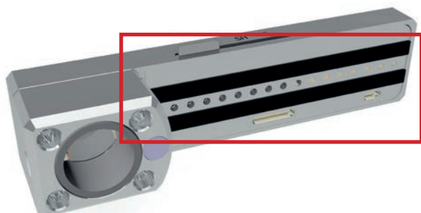
Pic. 9: Removing the microfibre stripes
