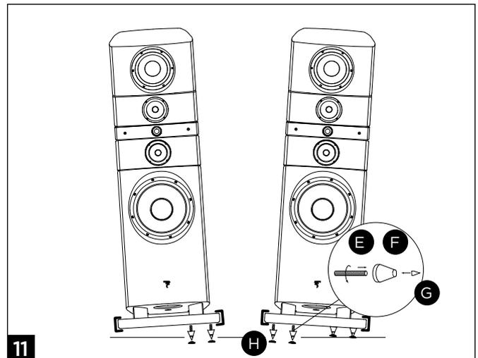
**Once the position is chosen, assemble ⑤, ⑥ and ⑦. To insert the spikes, lift the loudspeaker, one corner at the time (with the protection foams in place). Use the counter spikes ⑧ to protect the floor.**
