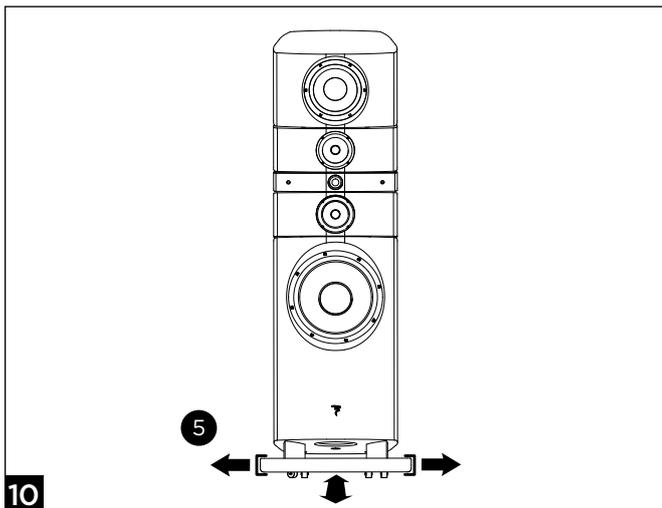
**You can move the loudspeakers to find the best place in the listening room. Leave the protection foams ⑤ in place.**
