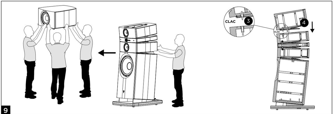
**Insert the 3 lugs ③ of the head in the holes of the body. Make sure that the rubber gasket ④ is well set up.**
